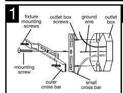
ATTACH small cross bar to outlet box with outlet box screws ( $8-32 \times 1/2$ , screws not provided). THREAD fixture mounting screws ( $8-32 \times 1,2$  provided) into large cross bar.
