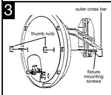
POSITION THE FIXTURE over the large cross bar and secure in place with the thumb nuts (2 provided). Screw bulb into socket. Be sure to use bulb with wattage no greater than specified for this fixture.
