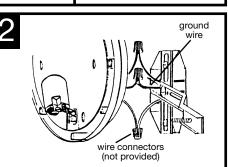
CONNECT THE WIRES. NOTE: Attach black fixture wire to black supply wire, white fixture wire to white supply wire. Do not mix them up. Use approved electrical tape or wire connectors (not provided). Connect bare fixture ground wire to ground wire from outlet box. NEVER CONNECT GROUND WIRE TO BLACK OR WHITE POWER SUPPLY WIRES.
